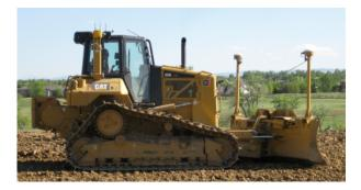
For finished grading work, with machine control the team was able to achieve finished grade to hundredths accuracy with fewer passes. Bulk excavation earthwork, utility trenching and foundations for the building were improved with the system because it measured the precise 3D position of the teeth of the bucket, turning the bulk earthmoving machine into a fine cutting and grading tool.
