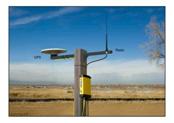
With a modular and flexible design, the SPS852 base station was mounted on the current Trimble building. It broadcasted on 900MHz and piped corrections to the Internet Base Station Service (IBSS) server for cellular connection.
